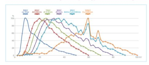
The SkyScan-1272 includes a 6-position automatic filter changer and is equipped with an X-ray source designed in such a way that adjustment of X-ray peak energy always keep the same output power. The flexibility for precise tuning of maximum X-ray energy emitted by the source and the minimum energy cut-off selected by numerous filters allows operator to select the most optimal energy window for any particular object. The control software can select best possible scanning protocol automatically.
