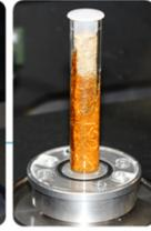
Optionally the system can be equipped with tube sample holders. A supplied set has four replaceable tube holders with plastic lids, which can be attached to a sealed baseplate. Tubes are 8 cm high, with internal diameters of (approx.) 6, 10, 15, 20 mm. The tube holders allow scanning samples with different sizes, including automated batch scanning, and imaging of hydrated samples and samples inside a liquid.
