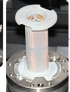
Another optional sample mount is dedicated to scanning several samples simultaneously for comparison. It contains two layers of parallel tube compartments for four samples up to 5mm in diameter in each layer. This allows analysis of 8 small samples - such as mouse bones, in a single scan.
