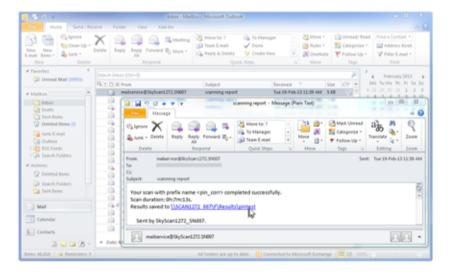
The SkyScan-1272 control software can send you an e-mail at the end of a scan. The e-mail contains a direct link to the data folder containing the scan results. By a simple click to this link one can open the dataset directly from a local computer. If the scanning process has been interrupted, the software will also email you a report of the details.
