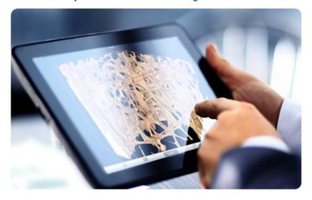
The CTVox, the volume rendering program supplied with the system, has a mobile version, which can be free downloaded from AppStore. Any 3D results obtained by the system can be send to a mobile device, such as iPad, for realistic visualization by real-time volume rendering with the possibility of 3D object manipulation, virtual cut, adjustments of object's opacity and colors, etc.
